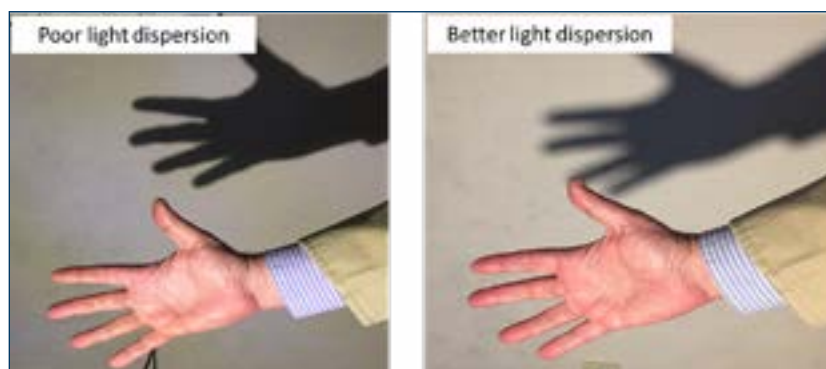
Figure 17. Some LED light sources produce light that is directional, creating sharp shadows which may attach unwanted nesting. Select light sources that produces diffuse light to reduce these shadows.
