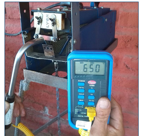
Pyrometer indicating proper blade temperature of 650°C.
